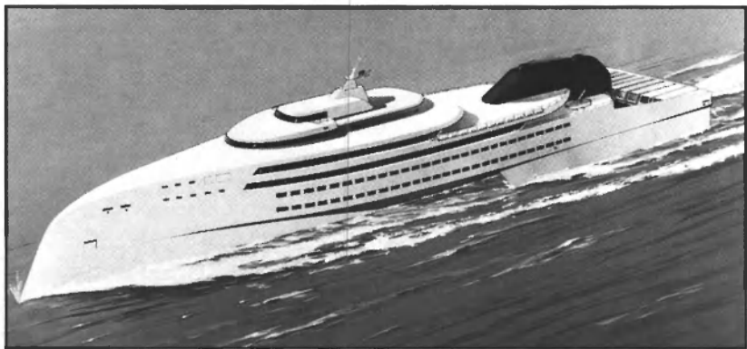
Trimaran HST-800: 40 Knot, Steel Trimaran, Gas Turbine, Passengers, Cars, Freight
