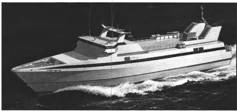
Monohull HSM-150: High Speed, Aluminum, Diesel, Passengers, Cars
