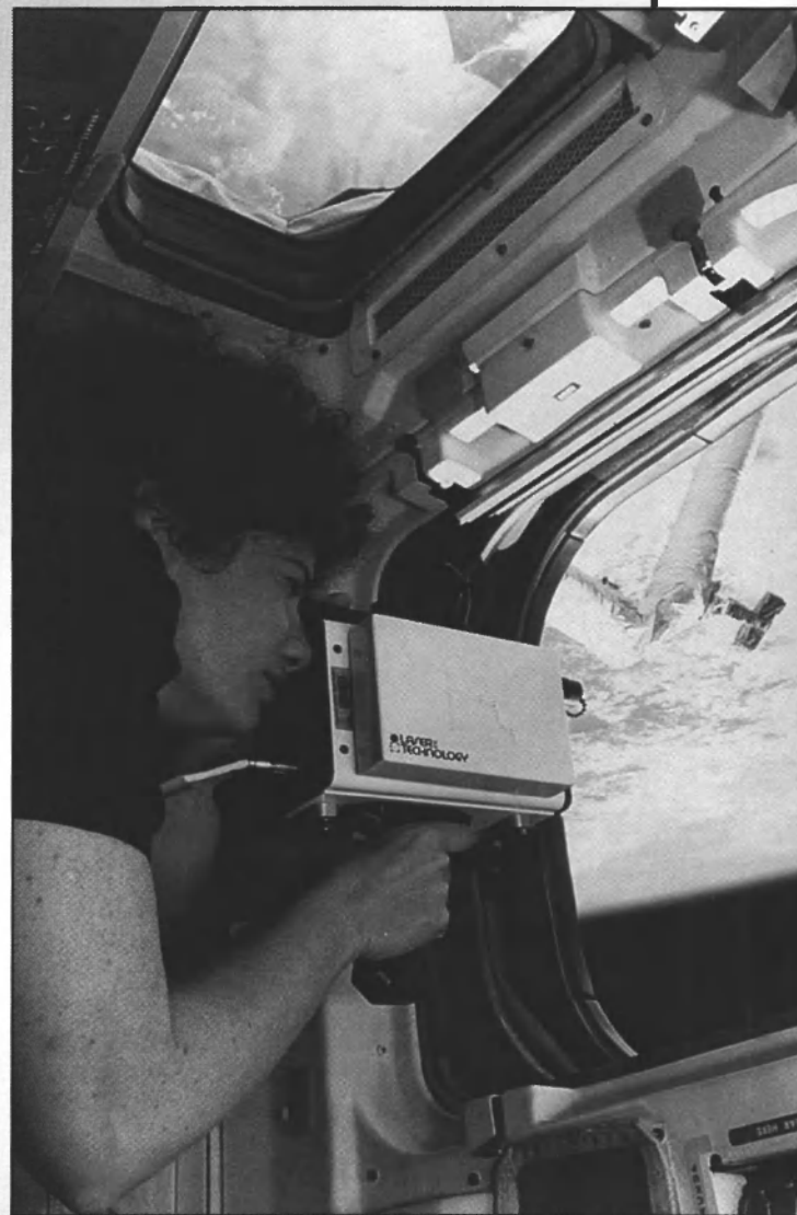
Laser Technology, Inc. designed and manufactured the laser docking system for NASA's astronauts to help dock the space shuttle with the Hubble Telescope and the Russian Mir in outer space.
