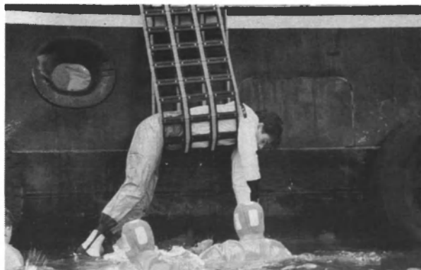
JASON'S CRADLE forms a par-buckle, giving the rescuer a 2:1 mechanical advantage. In most situations, once the casualty is placed in the non-collapsible loop, the recovery process takes 4-8 seconds
